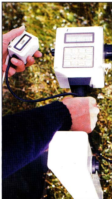
Figure 5. The Geoscan Research FM-36 fluxgate gradiometer as viewed by the operator. The fluxgate sensors are housed in the vertically oriented tube at the bottom of the photograph. The operator's left hand is holding a trigger device to activate an internal data logger.
